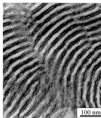
Fig. 7. TEM micrograph showing the morphology of a lamellar SBS star block copolymer having the same chemical composition as LN2-S74 (i.e. 74% volume fraction of PS) with PS domains in PB lamellae, OsO 4 staining.
